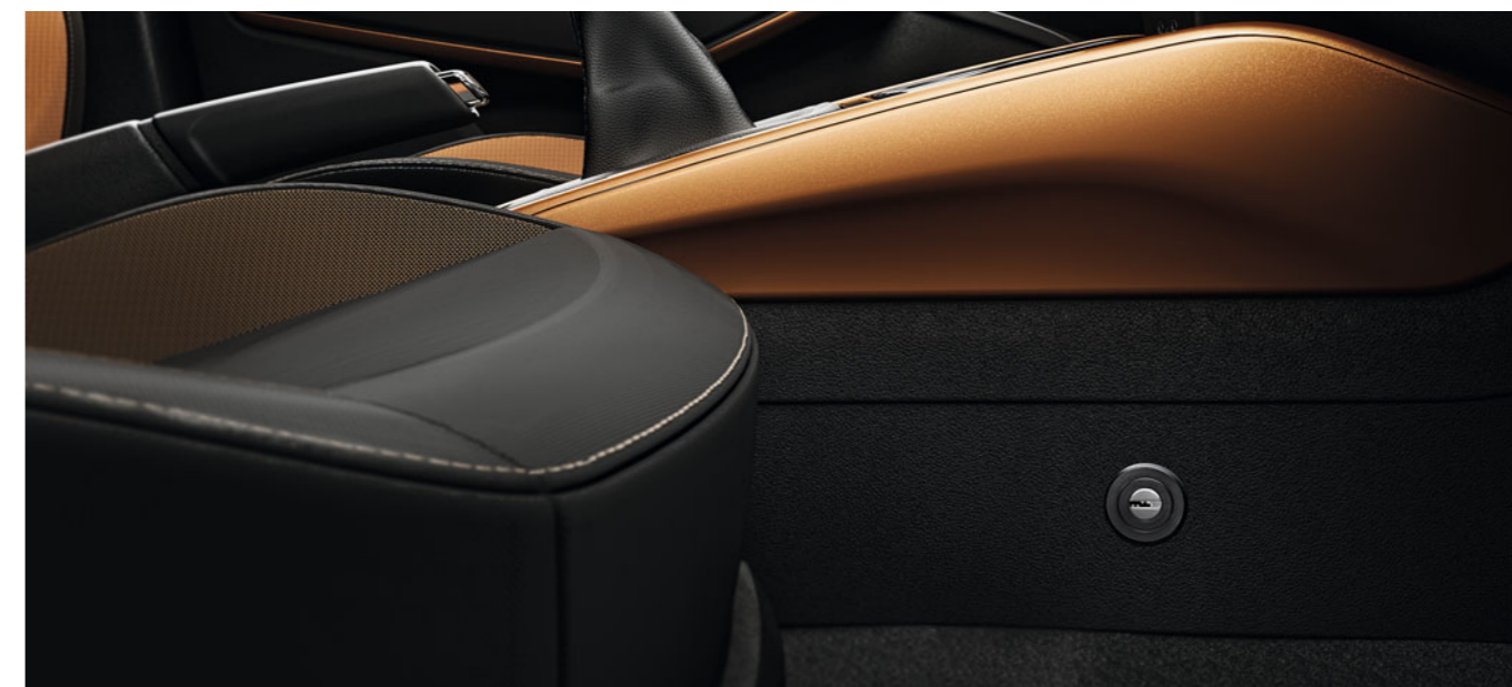
Mechanical gearbox locking system for LHD
