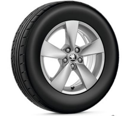
Hadar light-alloy wheel 5.5J x 15" ET40 for 185/65 R15 6VA 071 495 8Z8 | silver metallic
